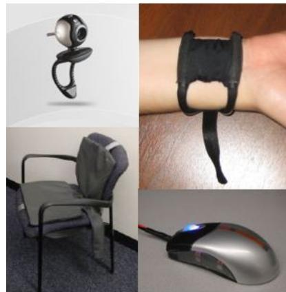
**Figure 1.** Sensors used in classrooms to detect student emotion; (clockwise) mental state camera, skin conductance bracelet, pressure sensitive mouse, and posture sensitive chair.
