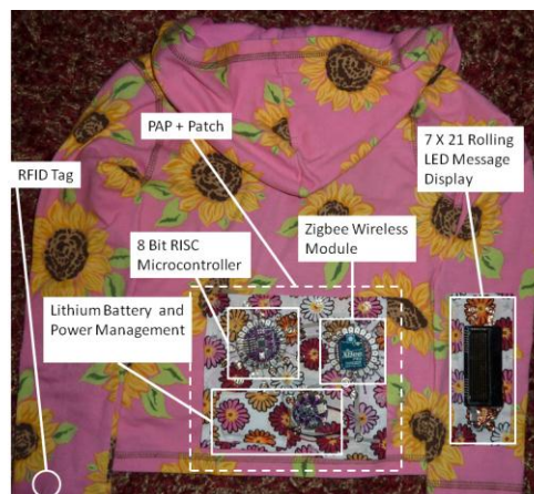
Figure 3. Wearable learning shirts (“hoodie”) provide electronic scaffolding for learning through children’s games, e.g. hide-and-seek and tag
