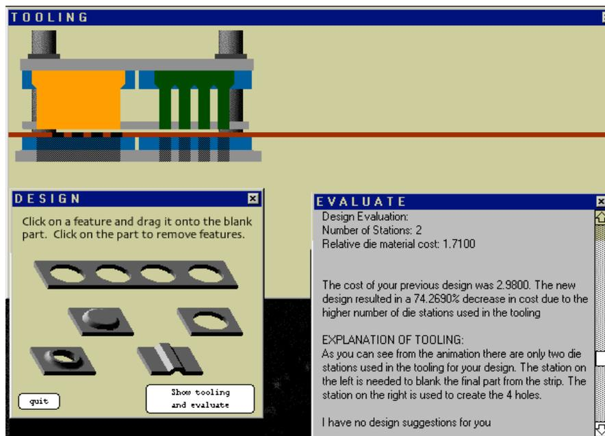
Figure 5. The strip redesigned as suggested by the evaluation shown in Fig. 4.
