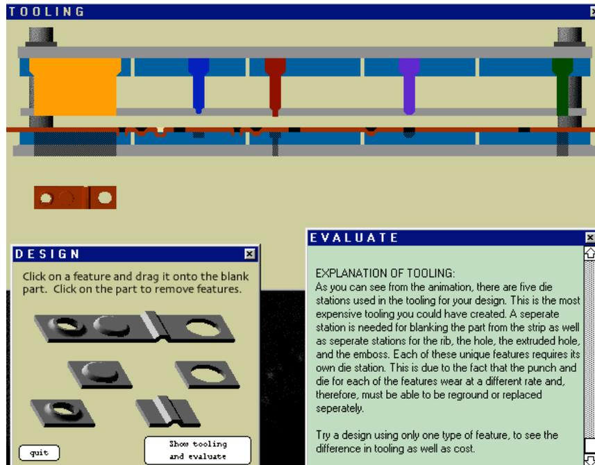
Figure 4. A snap shot from one of the workshop modules available for the stamping tutor. The tooling window contains an animated version of the five-station tool required to stamp the flat strip shown in the design window. An evaluation window is shown too.
