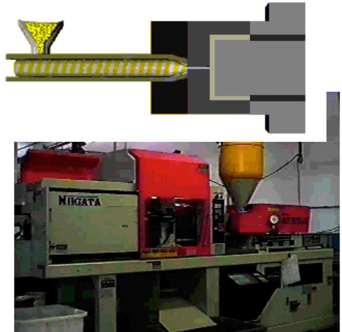
Figure 2. A snap shot of the animation showing an injection molding machine in its closed position. Text and the optional voice over explain that, "Injection molding is a common polymer process used to form thermoplastics, such as
