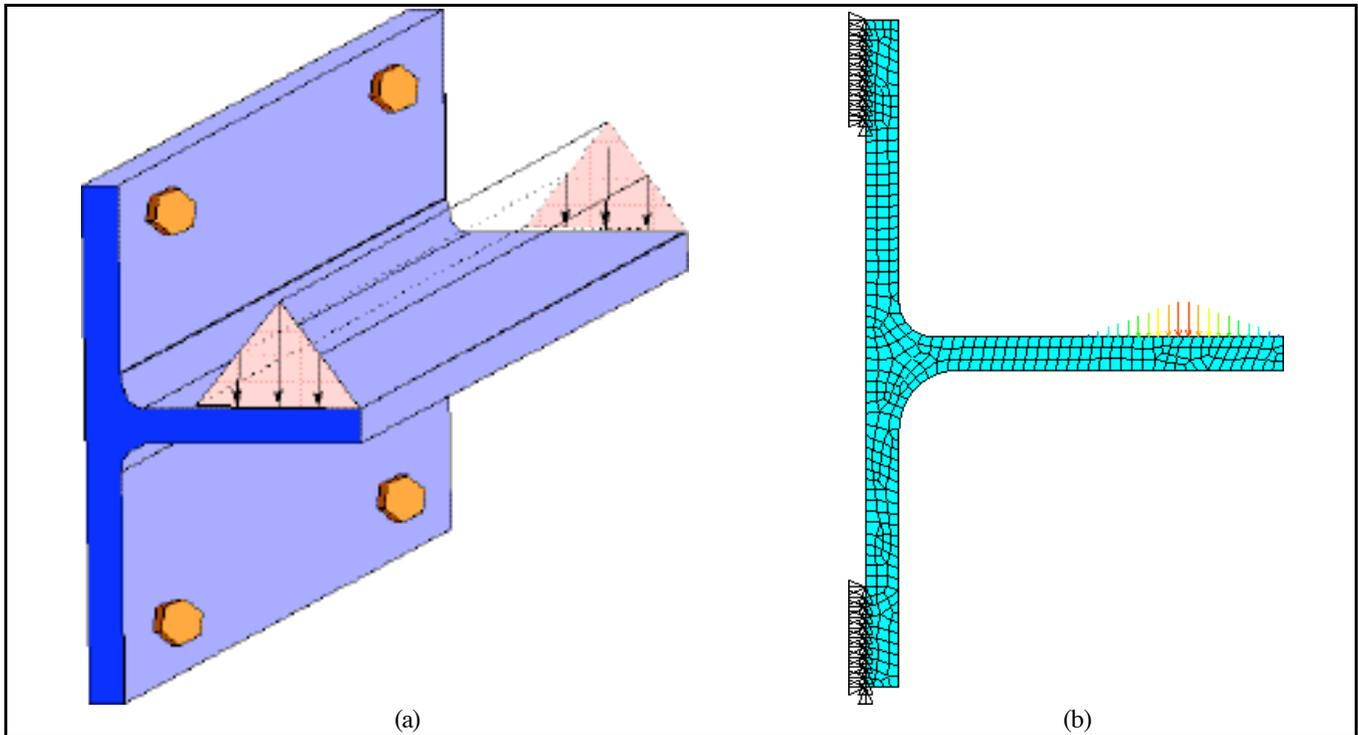
*Figure 6. The Tutor presents a student with predefined model (a), load and boundary conditions and ask for the necessary level of mesh refinement required (b).*
