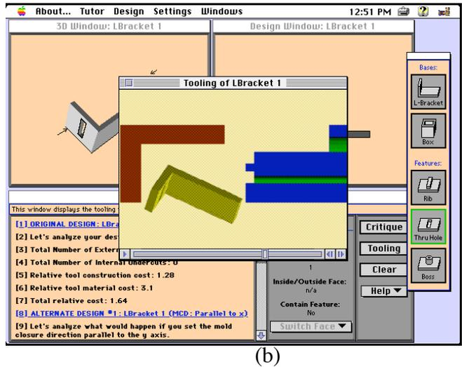
Figure 2. Critique (a) and tooling animation (b) for an L-bracket.
