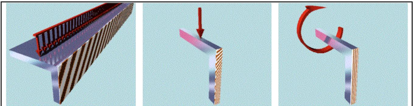
*Figure 5. The FEA Tutor teaches the basic concepts of model symmetry, load and boundary conditions and dimensional symmetry, including axisymmetry, plane stress and plane strain, and feature elimination.*
