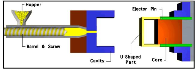
Figure 1. Injection Molding tooling required to produce a simple U-shaped part.
